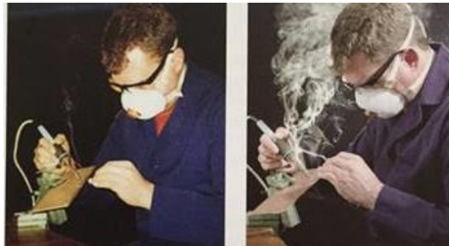
Soldering with and without Tyndall illumination
